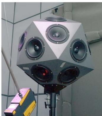
**Figure 40:** Laser Doppler vibrometry (LDV) measurements on an icosahedral loudspeaker array.
