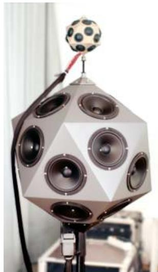
(b) IEM spherical loudspeakers, Graz
