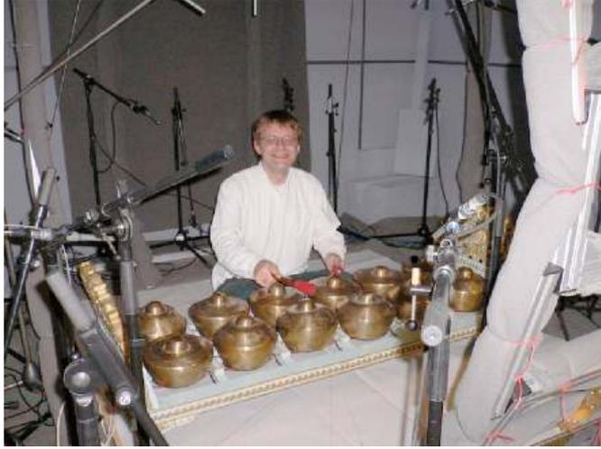
**Figure 3:** Capturing the sound-radiation of the *bonang barung* with 26 microphones in a hemispherical arrangement in an acoustically damped chamber at IEM (in the picture: Rainer Schütz (Institute of Ethnomusicology, Graz) playing it).
