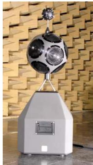
(c) ITA spherical loudspeakers, Aachen (photo: ITA, Behler)
