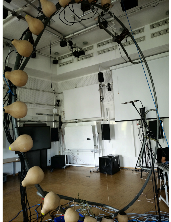
b) An Earthworks measurement microphone is used for the loudspeaker equalization.
