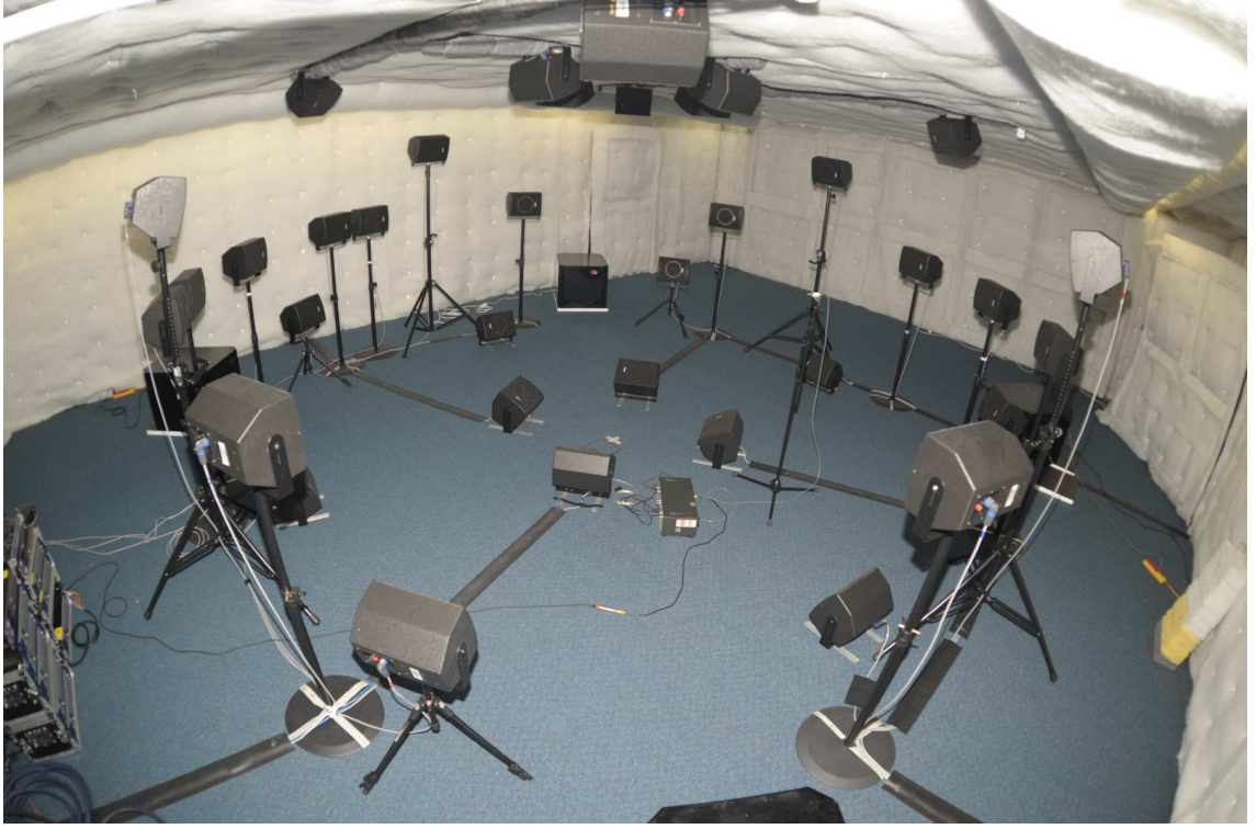
Figure 2: This figure shows a photo of the spherical loudspeaker array inside the hemi-anechoic room.
