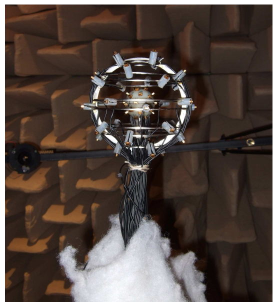
Figure 1: This figure shows a photo of the 64-microphone rigid and open spherical microphone array.
