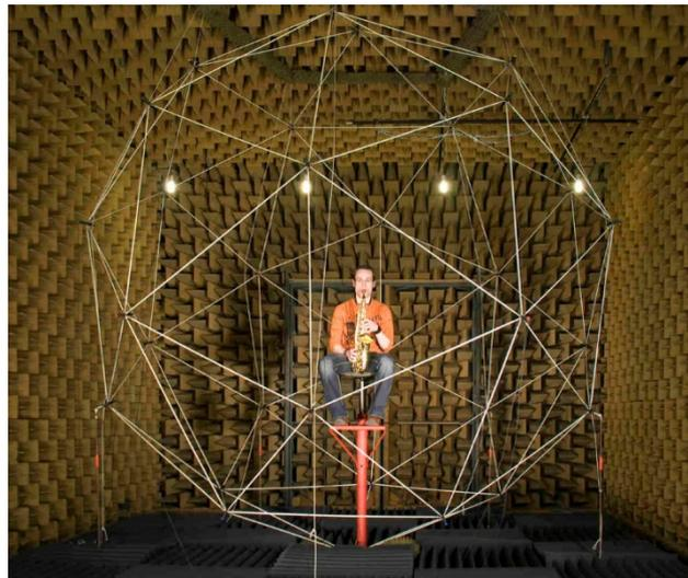
Figure 1: Spherical microphone array
