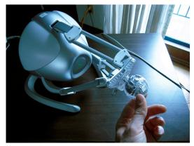
Figure 14: 3D force-feedback haptic controller
