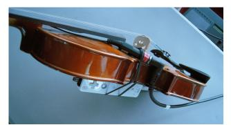
Figure 20: Violin with contact microphone and attached tilt-sensor
